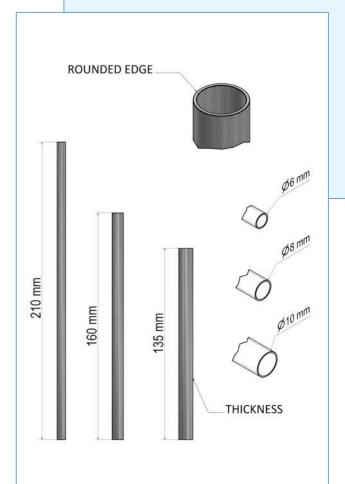
It is made of **AISI 316** stainless steel (18/8/3 austenitic and amagnetic steel), MARé is particularly resistant to corrosion from alkaline, acidic, alcoholic or corrosive drinks such as Coke, lemon-based drinks, sorbets and all drinks which contain high percentages of sugar.
